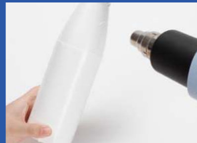
4. Heat the shrink film to make it fit tightly with the substrate;
